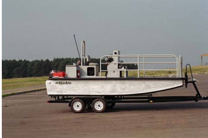
A custom designed barge for removing logjams was built and donated to the BBA by SEARK Marine, Inc. in Monticello, AR.
